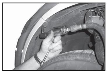
**4.** Remove one bolt on each side that connects facia to fender.
